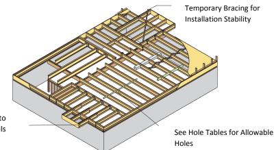
Reinforced Cantilever refer to Installation Details
